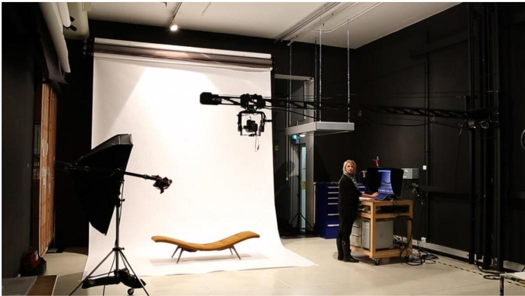
**The Zero G five axis Camera mount** is designed to allow the accurate positioning of a Video or stills camera anywhere within your studio space..... All with simple touch screen control. Repeatable positional accuracy of better than 1mm is achieved with the use of high precision DC servo motors, Zero backlash planetary gearheads and digital encoders. Full repeatable control of zoom and focus is also delivered.
